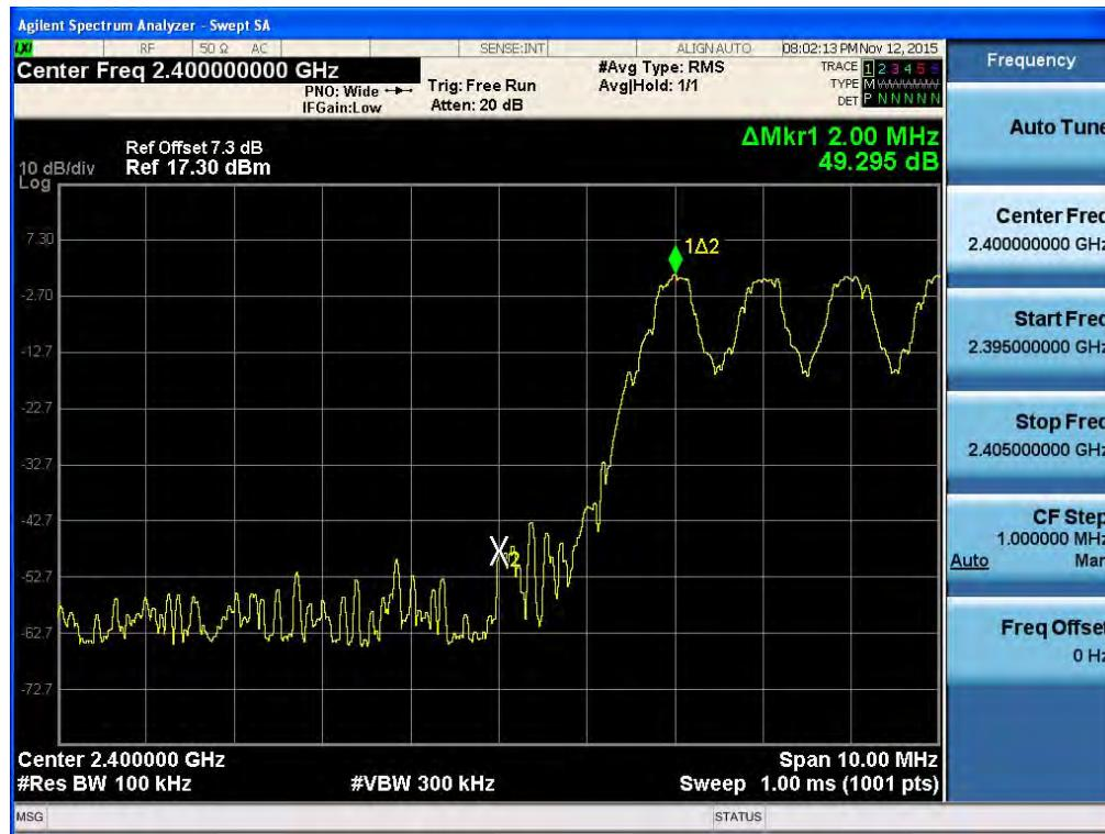
Test Plots with hopping (GFSK)
