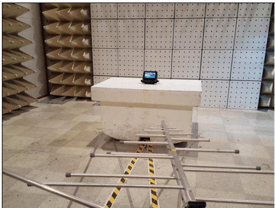
**3. Photo of Radiated Spurious Emission Test (Above 1 GHz)**
