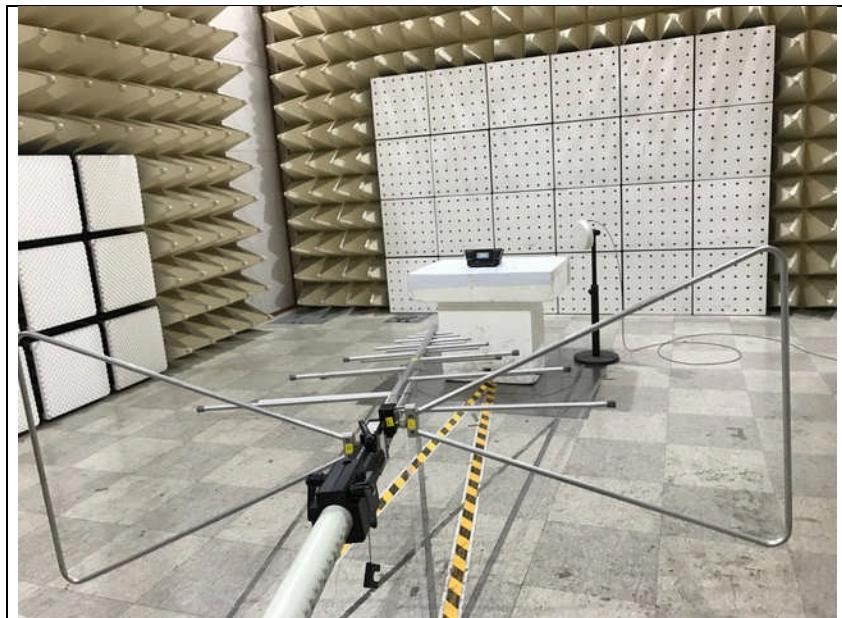
**3. Photo of Radiated Spurious Emission Test (Above 1 GHz)**
