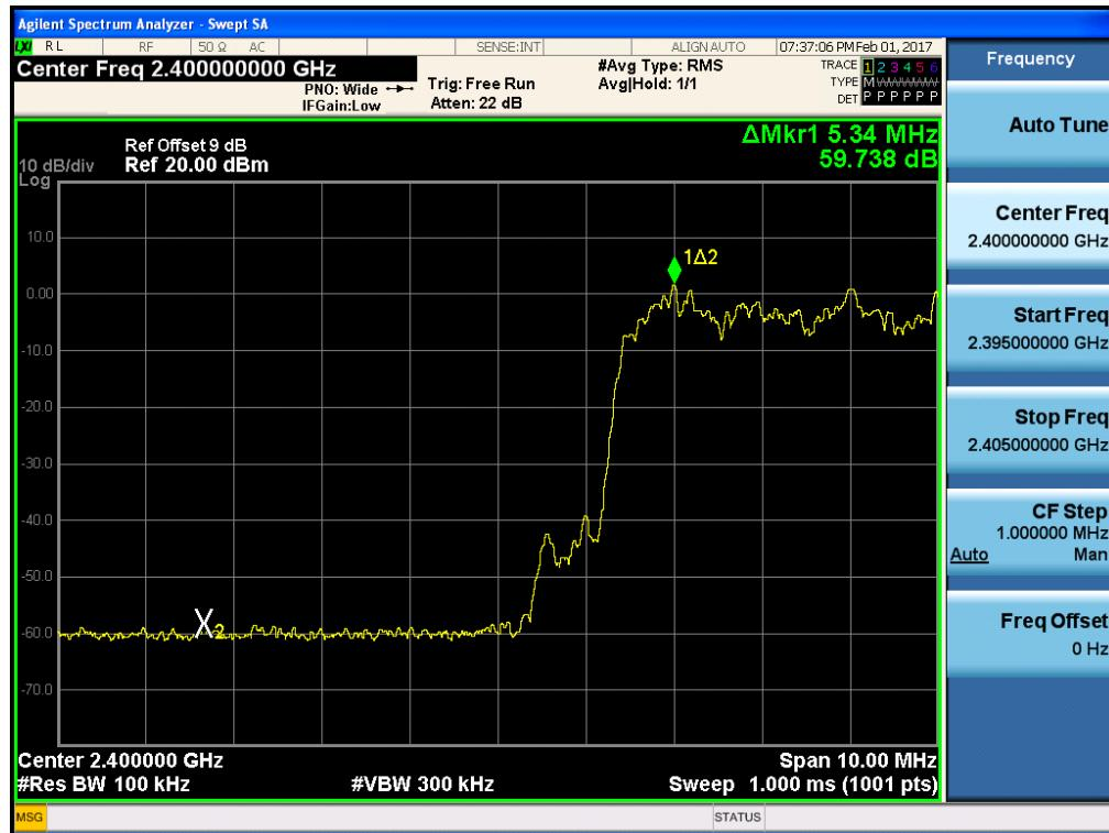
Test Plots with hopping (8DPSK)
