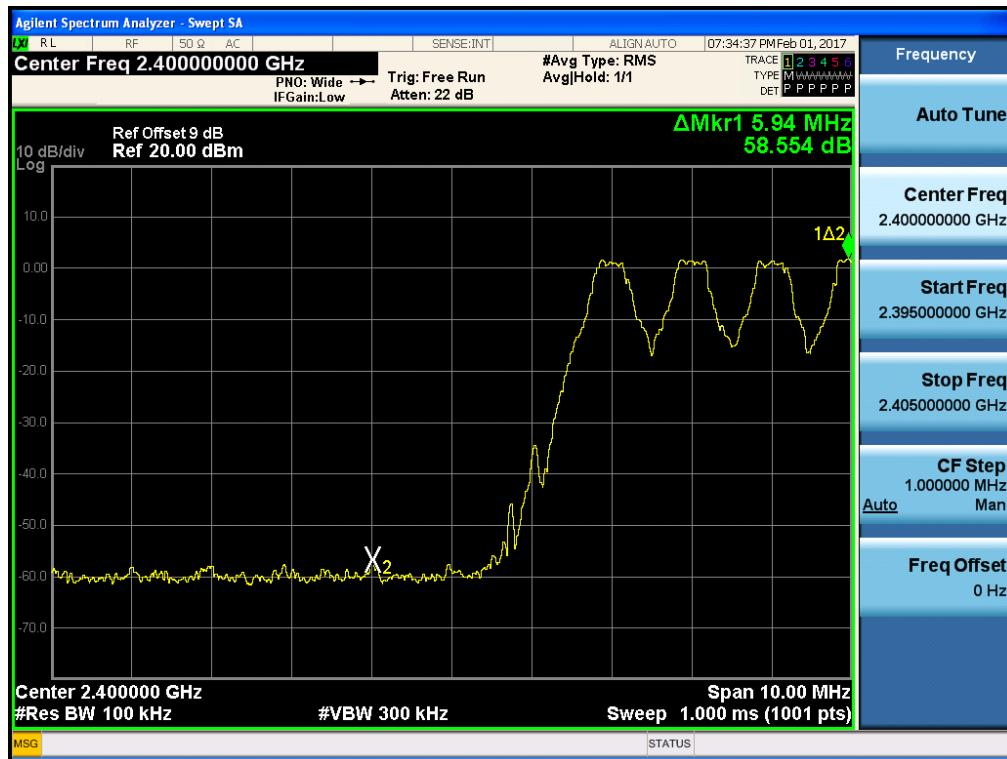
Test Plots with hopping (GFSK)
