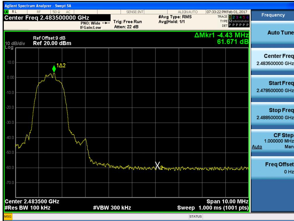
Test Plots with hopping (GFSK)
