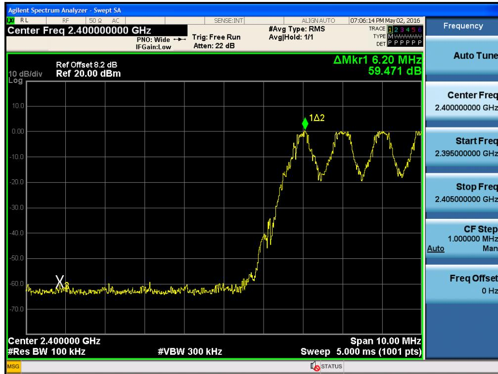
Test Plots with hopping (GFSK)
