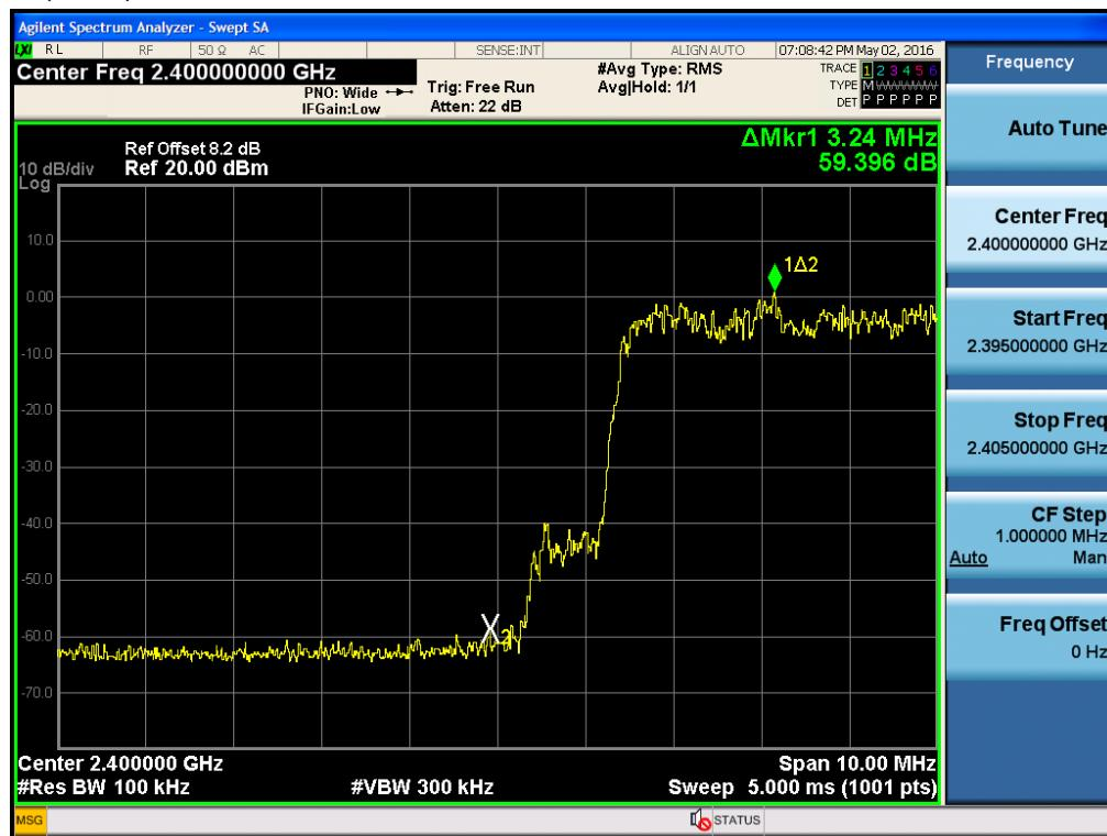
Test Plots with hopping (8DPSK)
