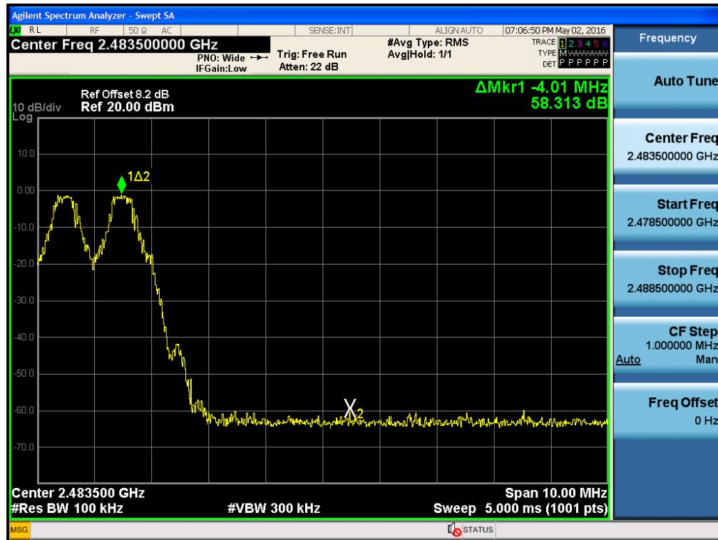
Test Plots with hopping (8DPSK)
