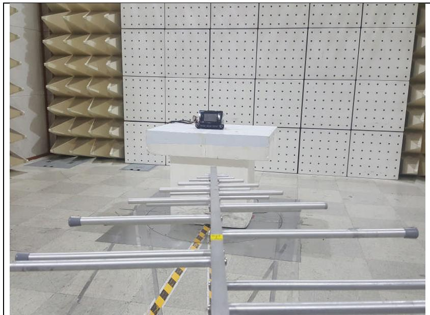
**3. Photo of Radiated Spurious Emission Test (Above 1 GHz)**
