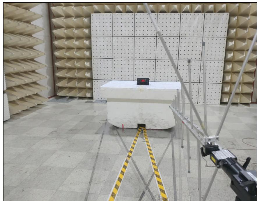
**2. Photo of Radiated Spurious Emission Test (Above 1 GHz)**
