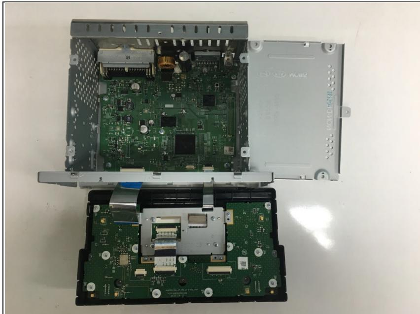
**Top view of main PCB**
