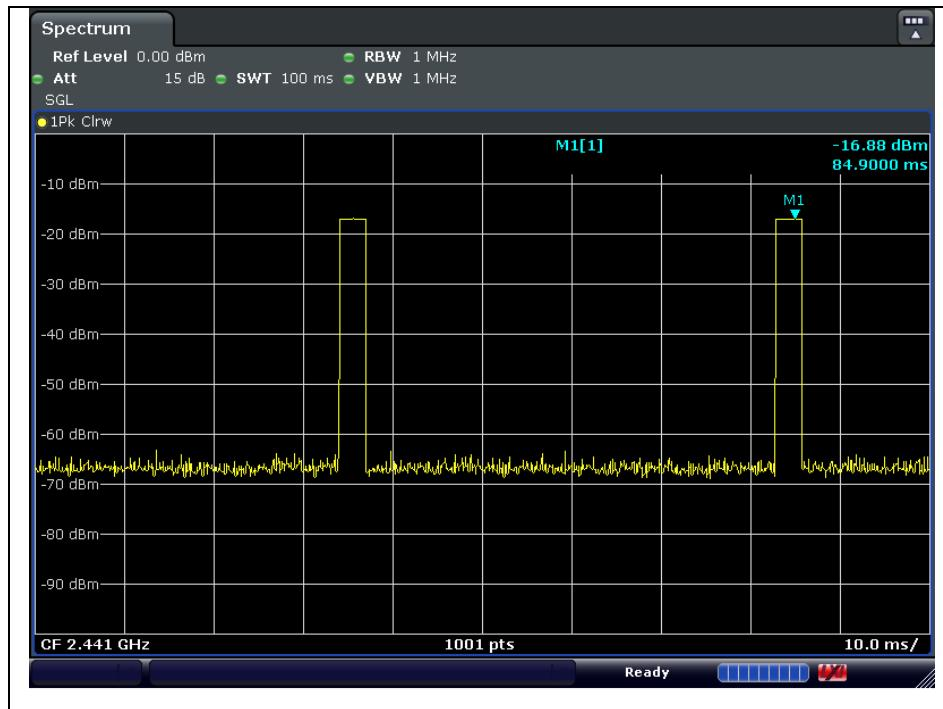
In AFH mode, the minimum hopping frequencies are 20, to get the longest dwell time DH5 packet is observed;
