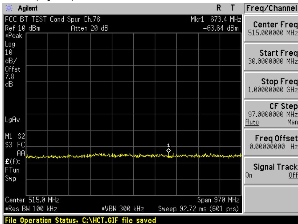
Test Plots (8DPSK) - 30 MHz - 1 GHz (RBW:100 kHz, VBW: 300 kHz)
