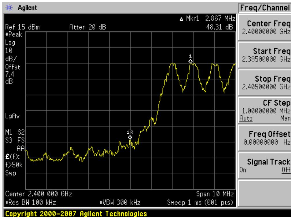
Test Plots with hopping (GFSK)
