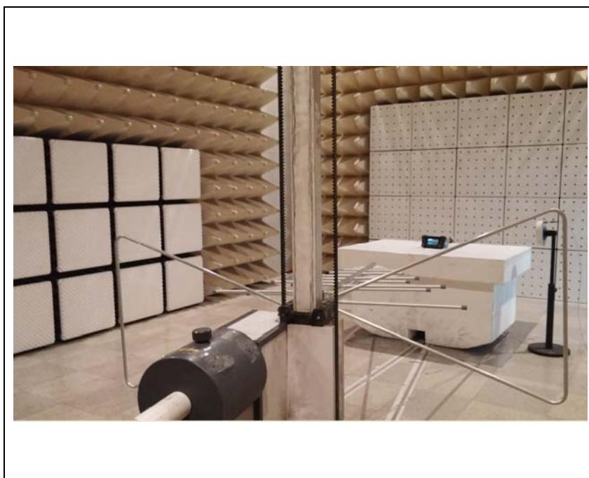
**B. Photo of Radiated Spurious Emission Test (Above 1GHz)**
