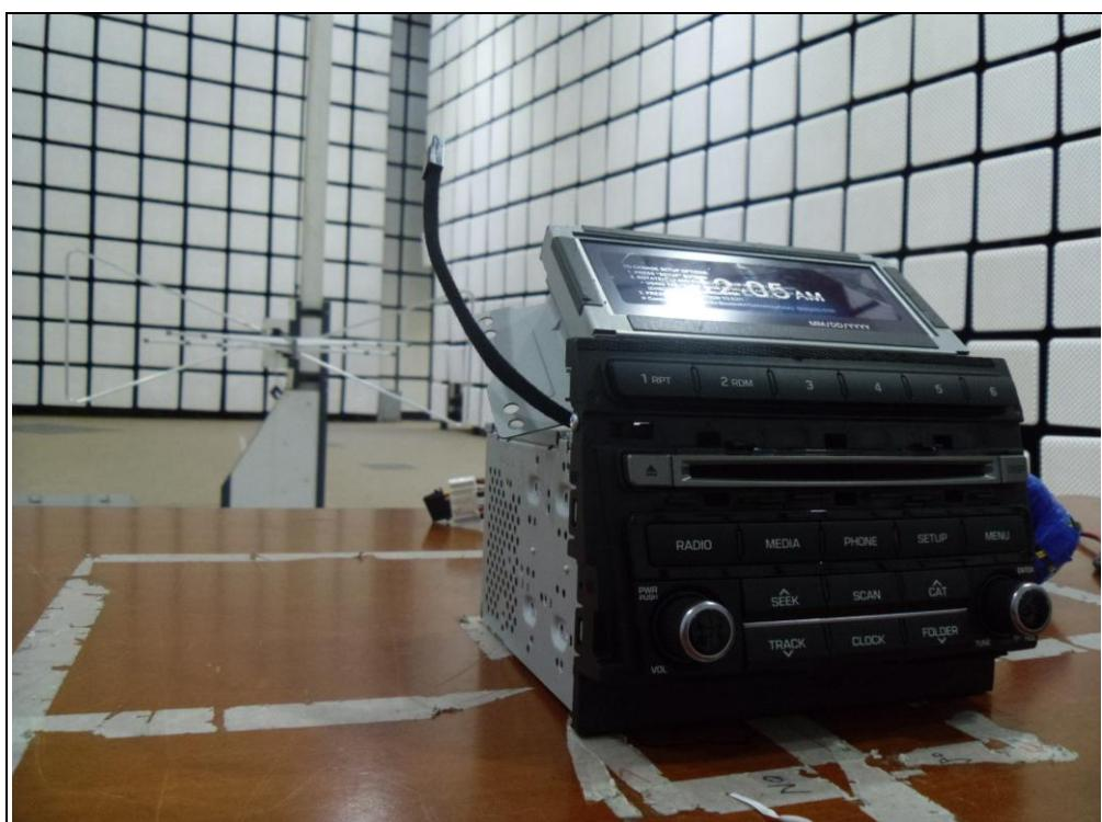
**C. Photo of Radiated Spurious Emission Test (Above 1 GHz)**
