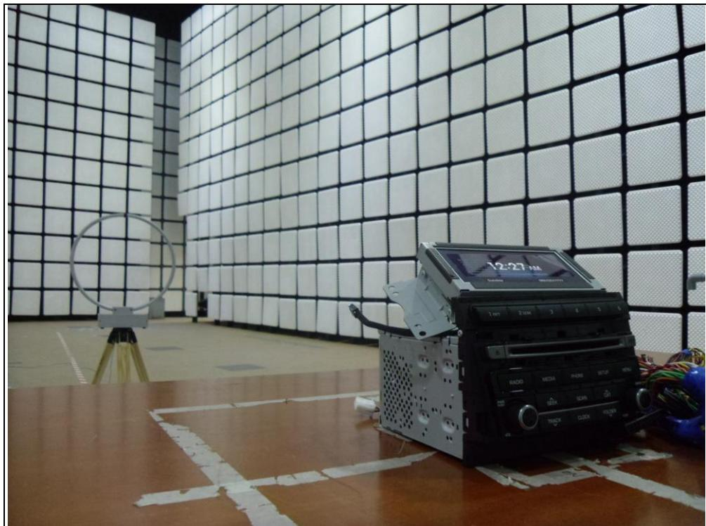
**B. Photo of Radiated Spurious Emission Test (30 MHz ~ 1 GHz)**
