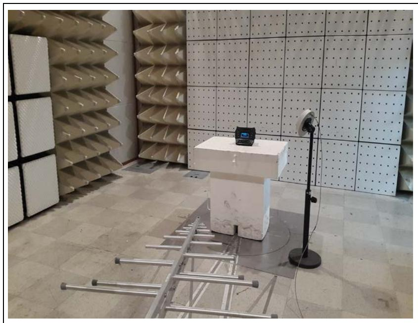
**B. Photo of Radiated Spurious Emission Test (Above 1 GHz)**
