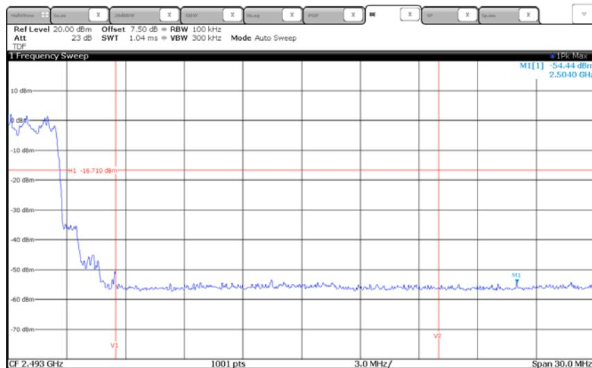
Figure 8. Plot of the Spurious RF conducted emissions
