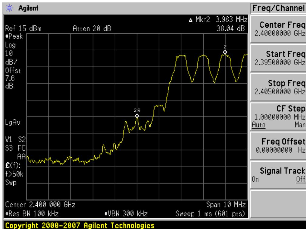
Test Plots with hopping (GFSK)
