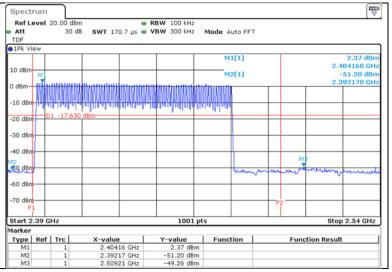
\* Result of 2 400.0 MHz - 2 483.5 MHz (F1: 2 400 MHz, F2: 2 500 MHz)
