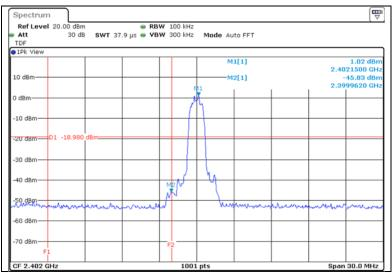
\* Result of 2 400.0 MHz (F1  $\sim$  F2: 2 390 MHz  $\sim$  2 400 MHz)
