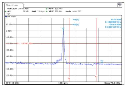
\* Result of 2 483.5 MHz (F1  $\sim$  F2: 2 483.5 MHz  $\sim$  2 500 MHz)
