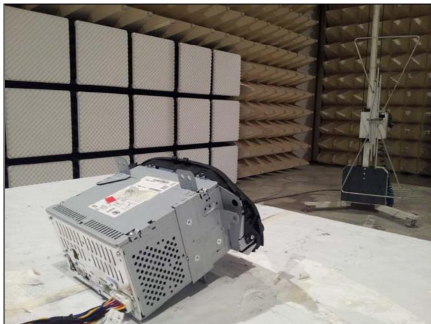
**C. E-Field and Radiated Emission (Horn Antenna)**
