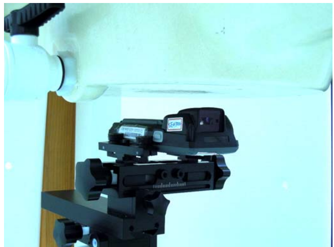
Rear Face of EUT with 1.5 cm Gap (EUT Standalone)
