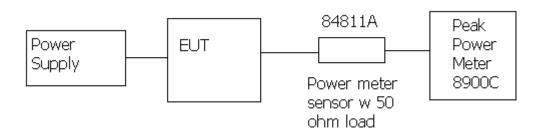
POWER OUPUT: 39 mW (0.039 Watts) meets the FCC requirements.
