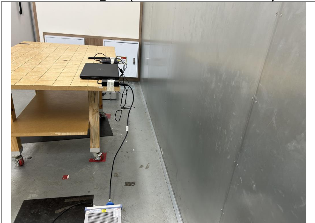
Conducted Emission_Rear (Worst Case : External Antenna)
