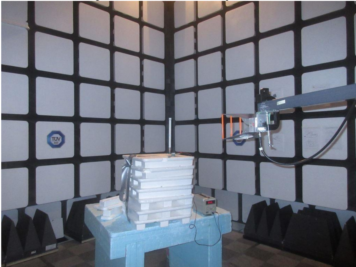
Figure 3 – Radiated Emissions Setup – Photo 3
