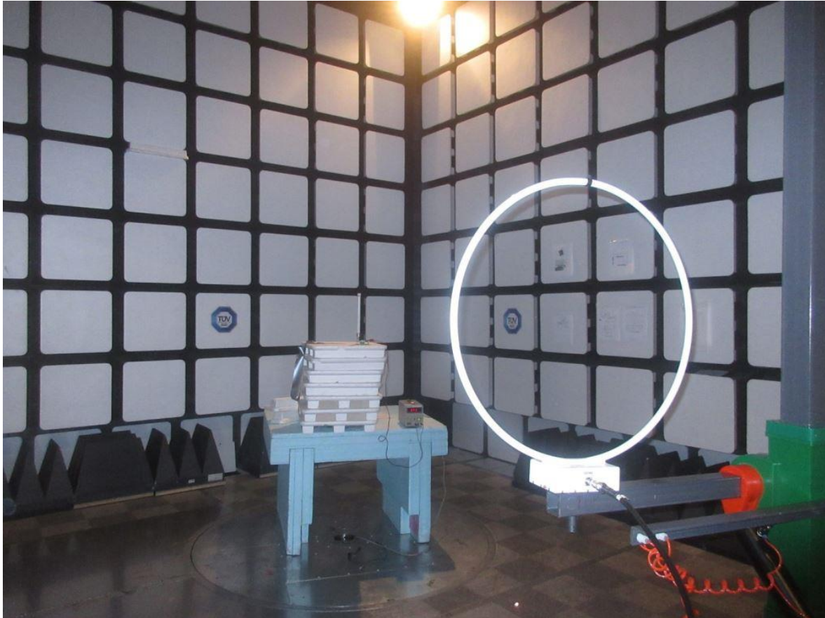
Figure 1 – Radiated Emissions Setup – Photo 1
