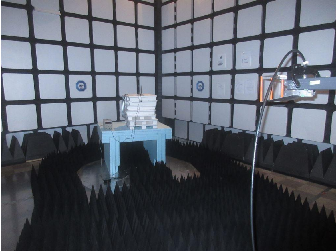
Figure 4 – Radiated Emissions Setup – Photo 4
