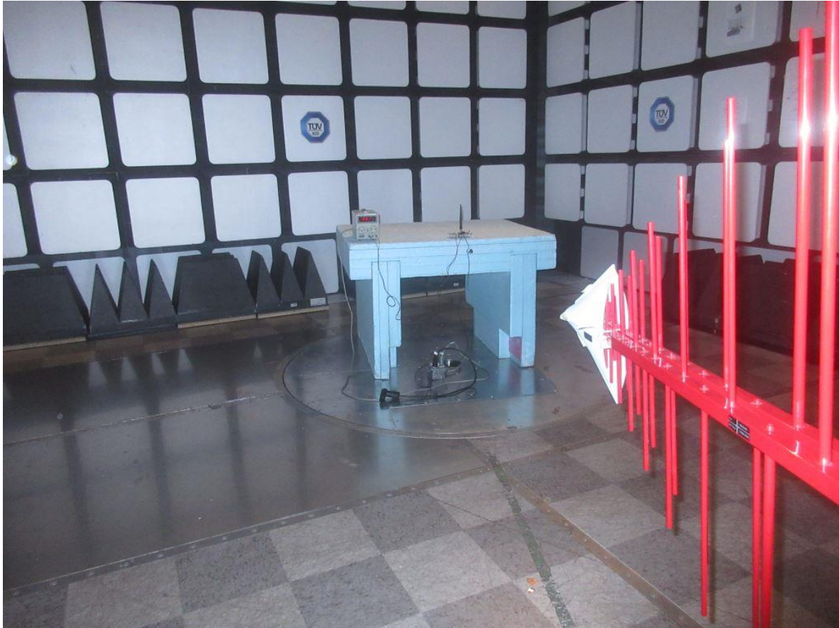
Figure 2 – Radiated Emissions Setup – Photo 2
