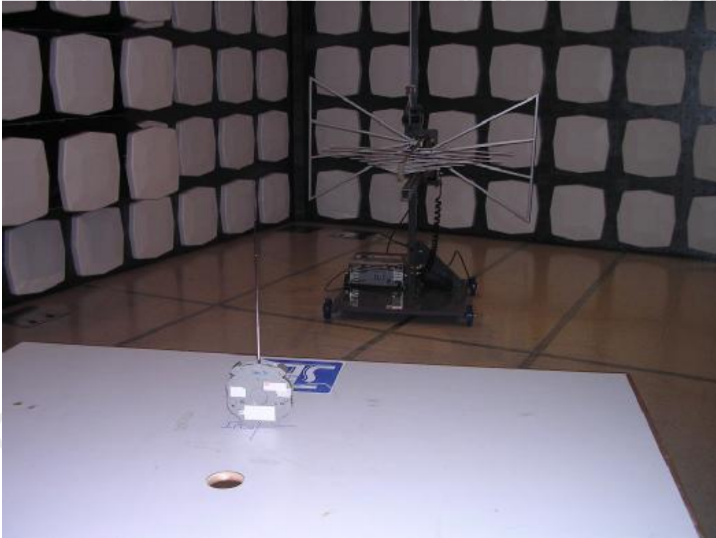
Measurement of Radiated Emission Test Set Up
