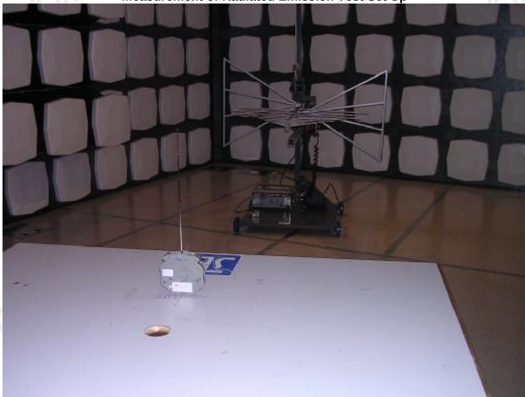
Measurement of Radiated Emission Test Set Up
