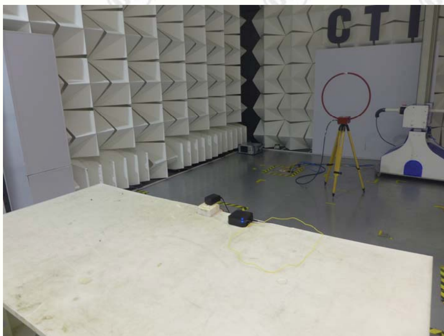
Radiated emission Test Setup-2(9kHz~30MHz)
