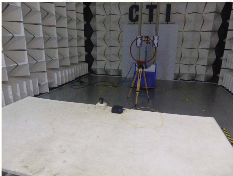
Radiated emission Test Setup-1(9kHz~30MHz)
