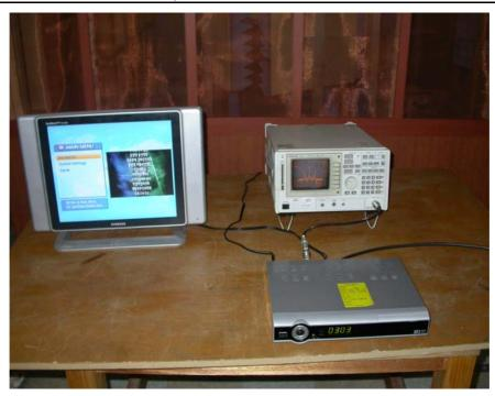
Setup for Output signal conducted level
