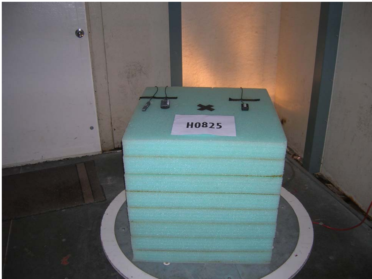
Radiated Emissions Setup Receiver shown with Head Tracker Transmitter for communications.
