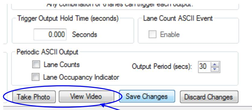
Click the "Take Photo" button to take a snapshot of the radar view of the road. This is a very convenient feature of the PX150 to verify proper pointing both in the vertical and horizontal direction. Ensure you are pointed as close to 90° to the passing traffic as possible for best results.
