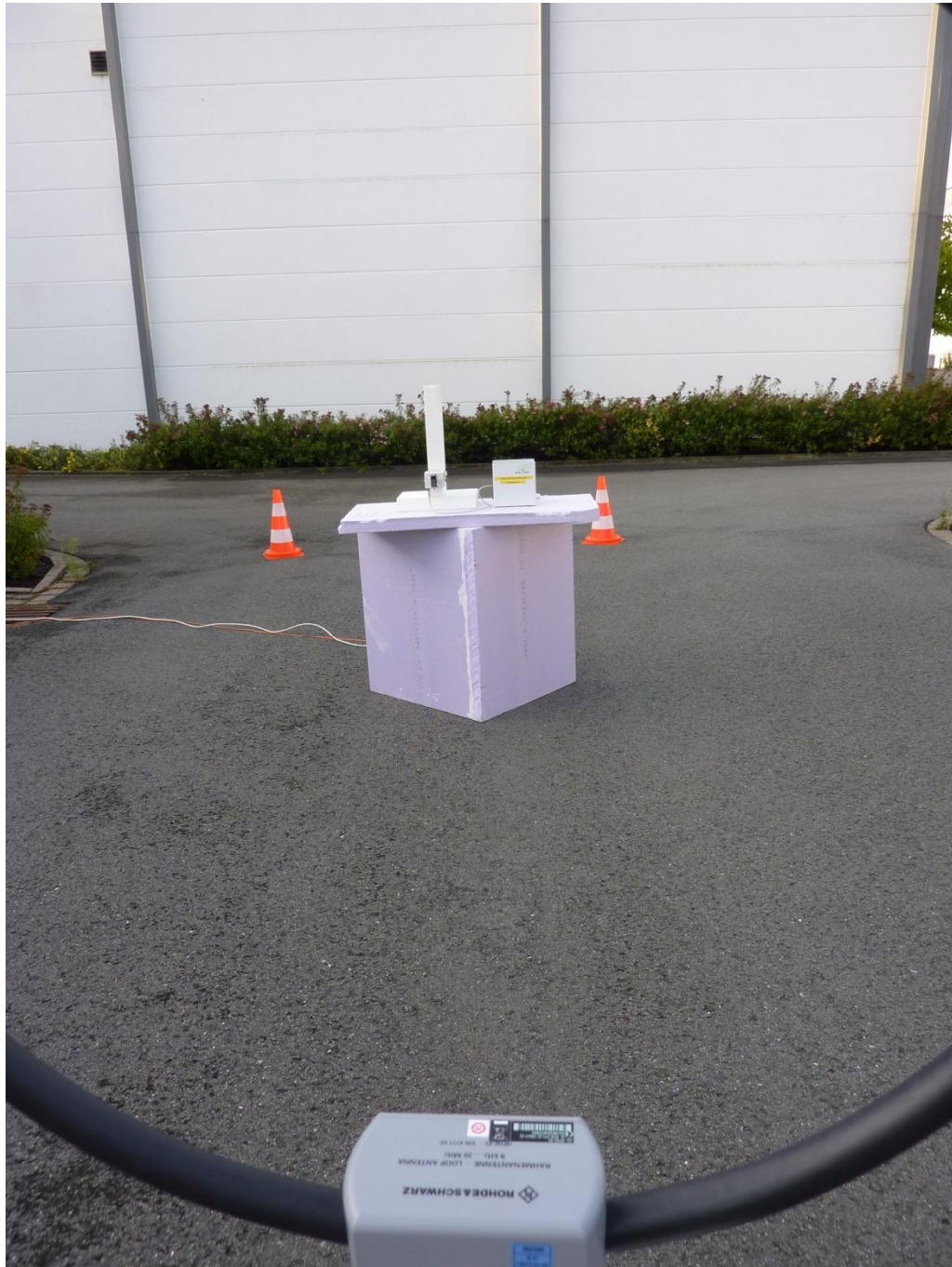
161006_1e.jpg: QXL45 Liquid Dosing Module, test setup outdoor test site
