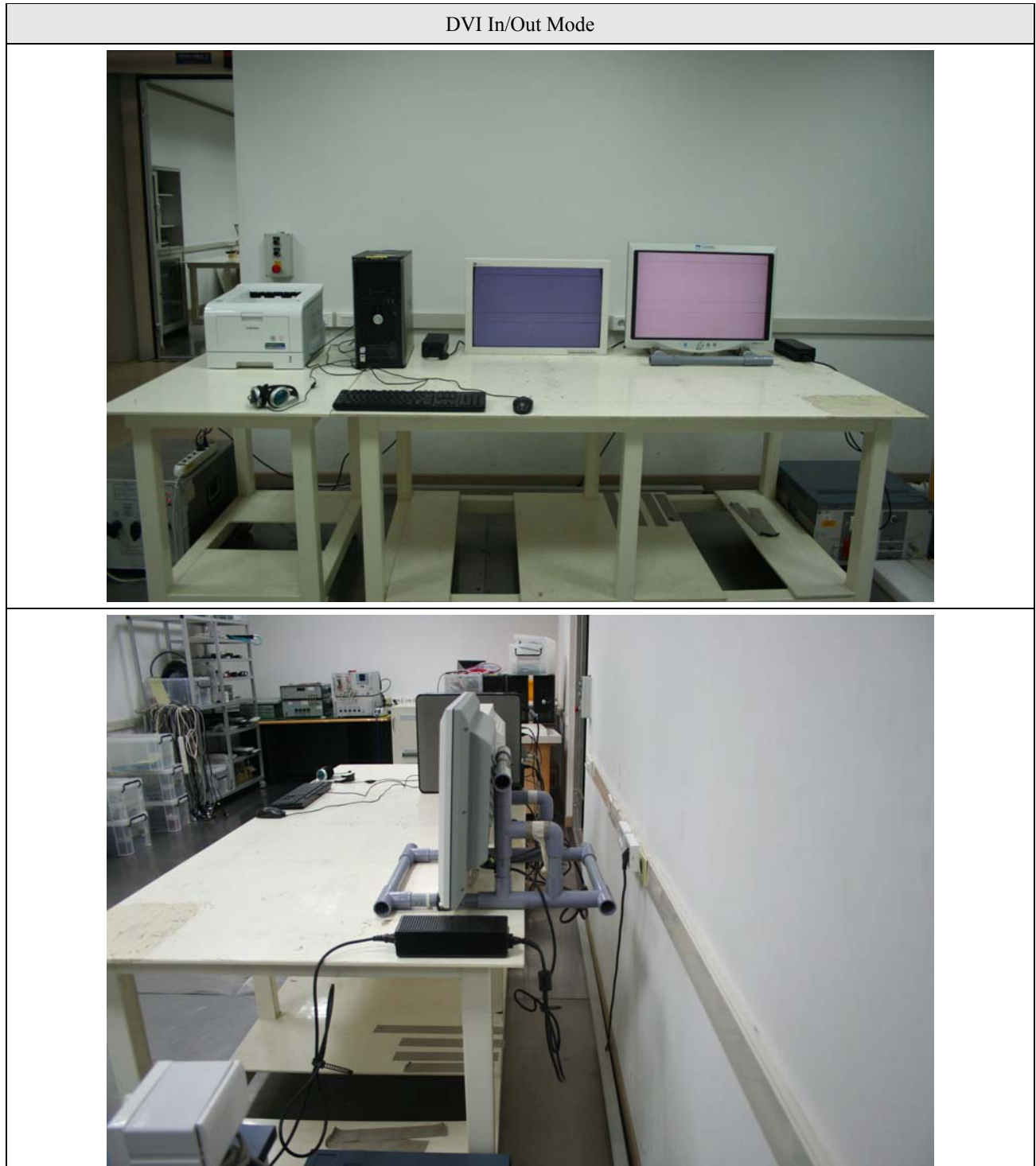
Figure 1. Conducted Emission Test Setup
