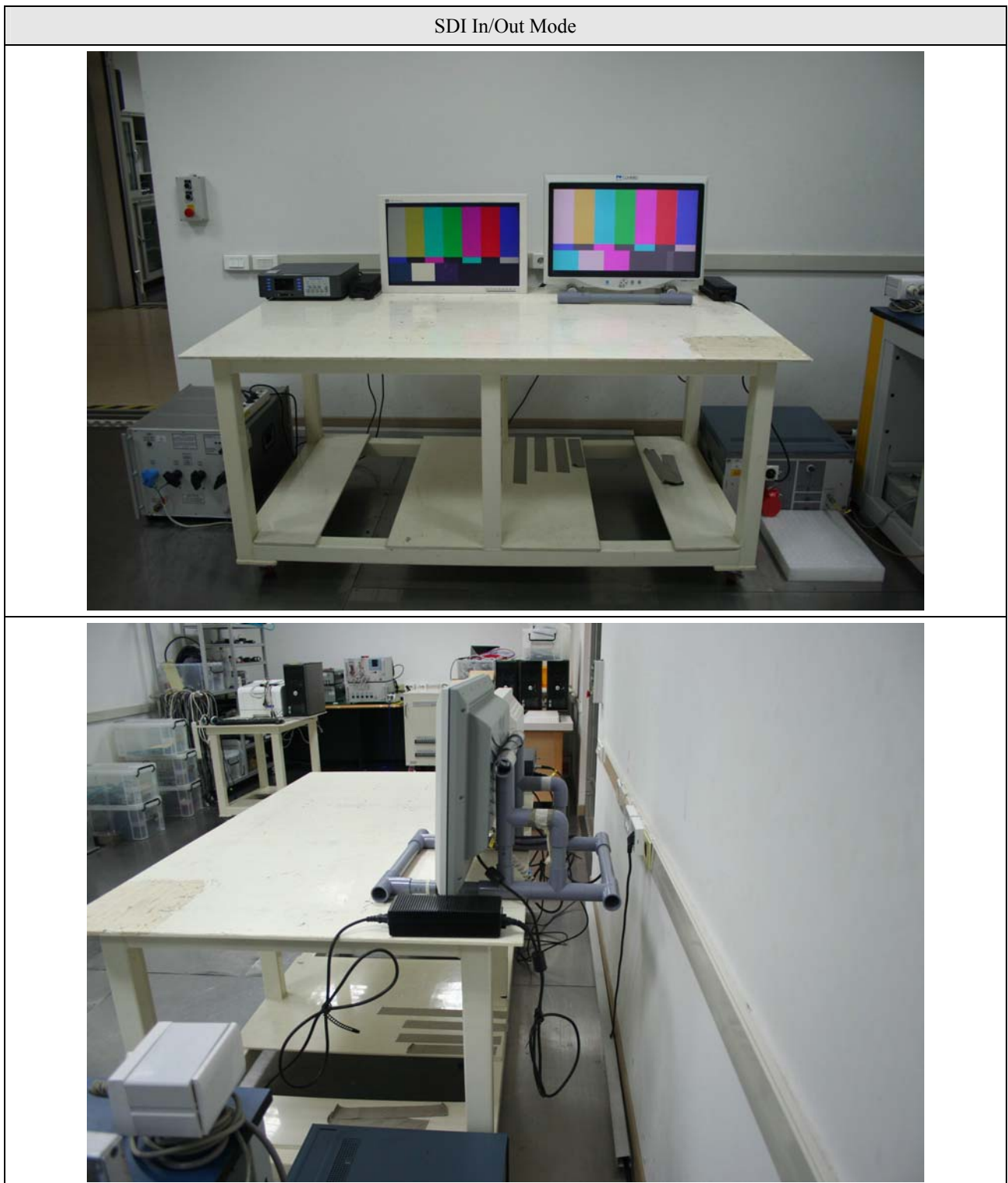
Figure 3. Conducted Emission Test Setup
