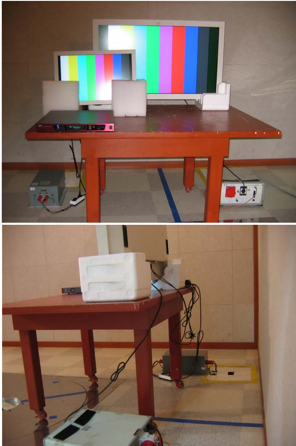
Figure 2 Conducted Emission Test Setup: SDI Mode
