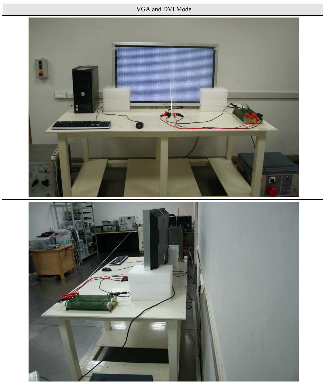
Figure 1. Conducted Emission Test Setup
