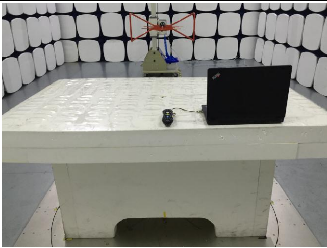
Radiated Spurious Emissions Test Setup Below 1GHz
