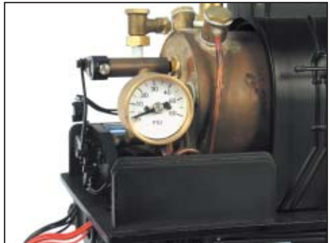
fig. #20a Locomotive pressure gauge
