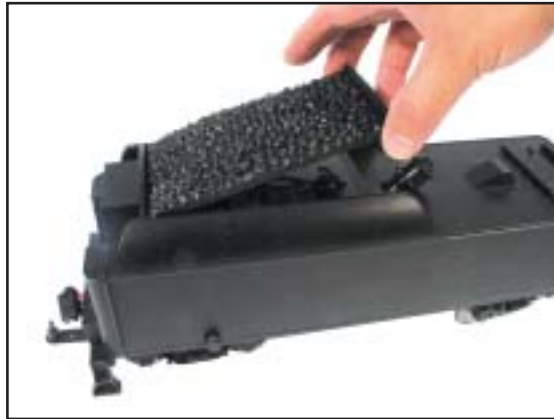
fig. #21 Replacing the coal load
