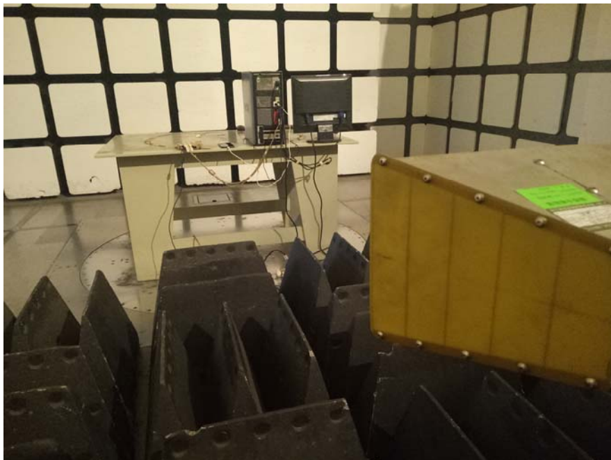
Radiated Emissions – Rear View (Above 1 GHz)
