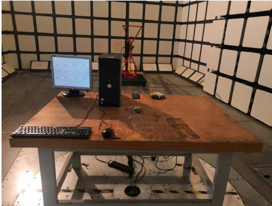
Radiated Emissions – Front View (Below 1 GHz)
