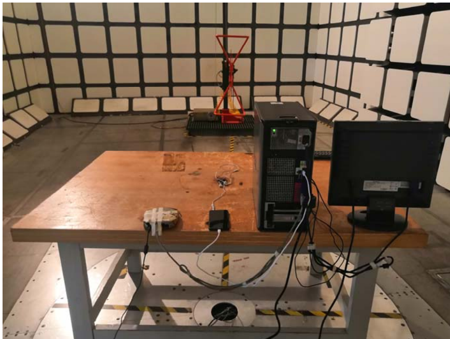
Radiated Emissions – Rear View (Below 1 GHz)
