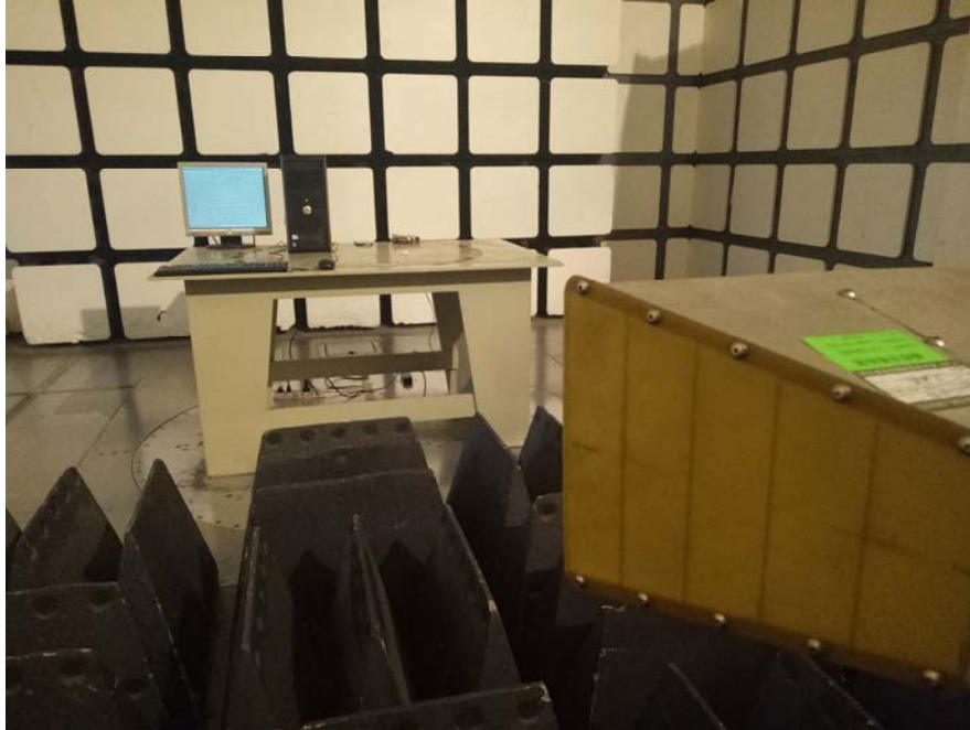
Radiated Emissions – Front View (Above 1 GHz)
