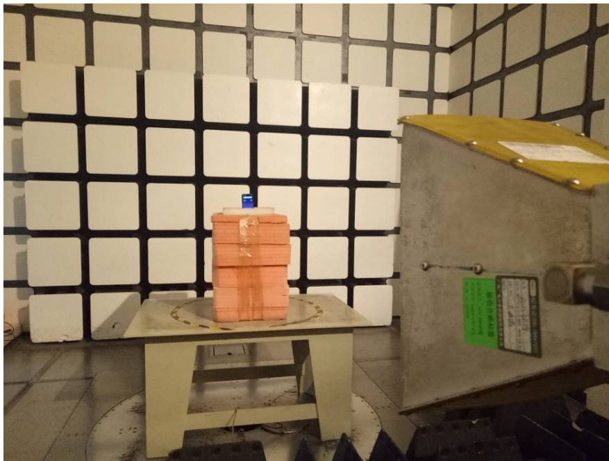
Radiated Emissions View (Above 1 GHz)
