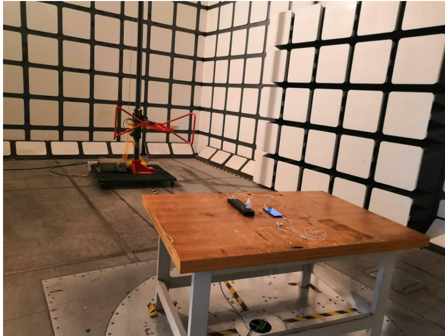
Radiated Emissions View (Below 1 GHz)
