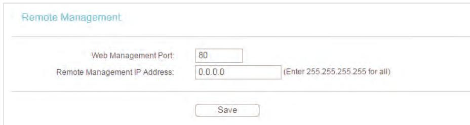
The image shows a screenshot of a web-based configuration interface for a router. The page is titled 'Remote Management'. It contains two main input fields: 'Web Management Port' with the value '80' and 'Remote Management IP Address' with the value '0.0.0.0'. A note next to the IP address field says '(Enter 255.255.255.255 for all)'. At the bottom of the form is a 'Save' button.
