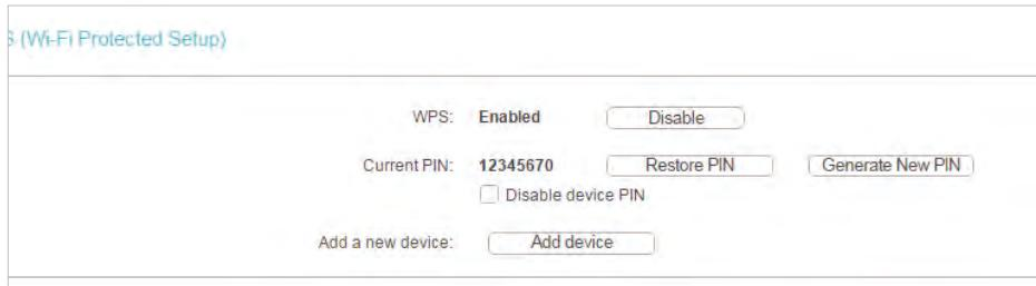
The screenshot shows the 'Wi-Fi Protected Setup' configuration page. The 'WPS' status is set to 'Enabled' with a 'Disable' button. The 'Current PIN' is displayed as '12345670' with 'Restore PIN' and 'Generate New PIN' buttons. A checkbox for 'Disable device PIN' is present. At the bottom, there is a 'Add a new device:' field and an 'Add device' button.
