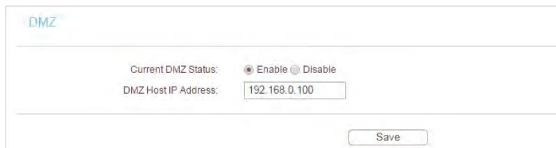
The screenshot shows a configuration page for a DMZ host. At the top, it says 'DMZ'. Below that, there are two radio buttons for 'Current DMZ Status': 'Enable' (which is selected) and 'Disable'. Underneath is a 'DMZ Host IP Address' field containing '192.168.0.100'. At the bottom right of the form is a 'Save' button.
