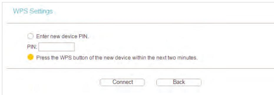
The screenshot shows the 'WPS Settings' page. It provides two methods for connection: 'Enter new device PIN' (radio button selected) and 'Press the WPS button of the new device within the next two minutes' (radio button unselected). Below these options are 'Connect' and 'Back' buttons.
