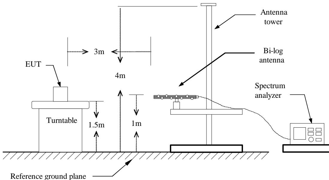
**Above 1 GHz**
