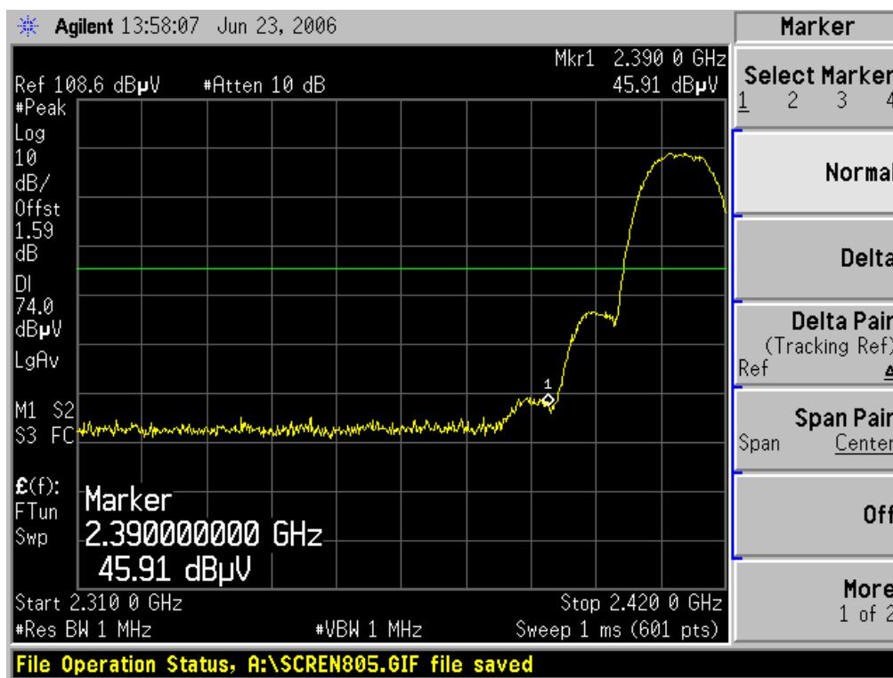
**Detector mode: Average****Polarity: Vertical**
