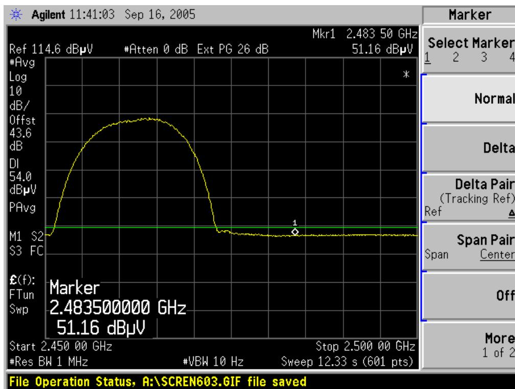
**Band Edges (802.11g / CH Low)****Detector mode: Peak****Polarity: Vertical**
