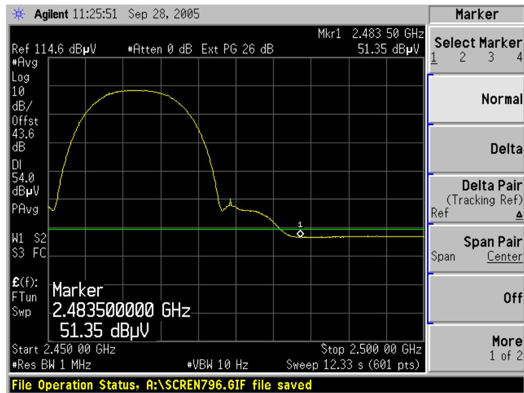
**Band Edges (802.11g / CH Low)****Detector mode: Peak****Polarity: Vertical**
