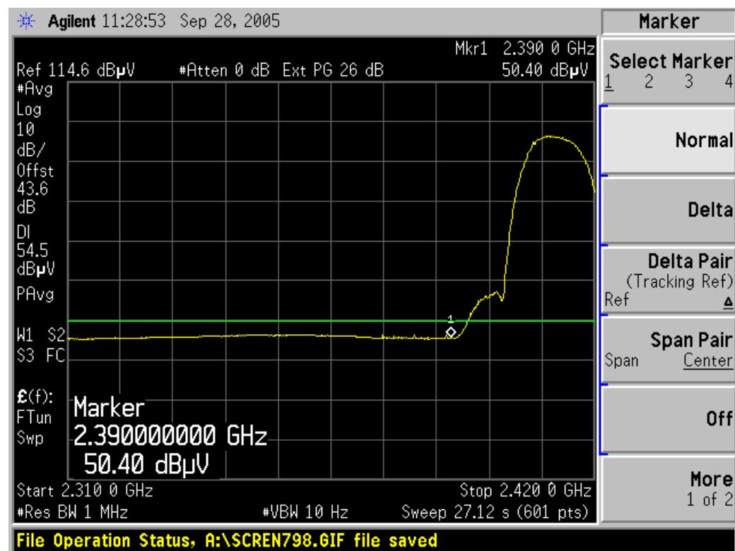
**Band Edges (802.11b / CH High)****Detector mode: Peak****Polarity: Vertical**
