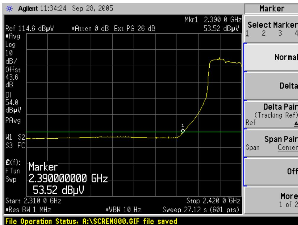
**Band Edges (802.11g / CH High)****Detector mode: Peak****Polarity: Vertical**
