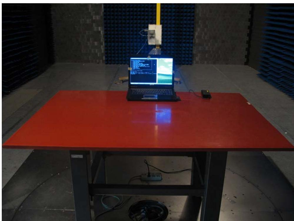
Test Mode: Mode 2: Transmit by 802.11g
