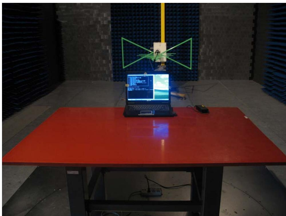
Test Mode: Mode 1: Transmit by 802.11b
