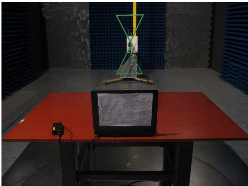
Test Mode: Mode 1: Transmit by 802.11b
