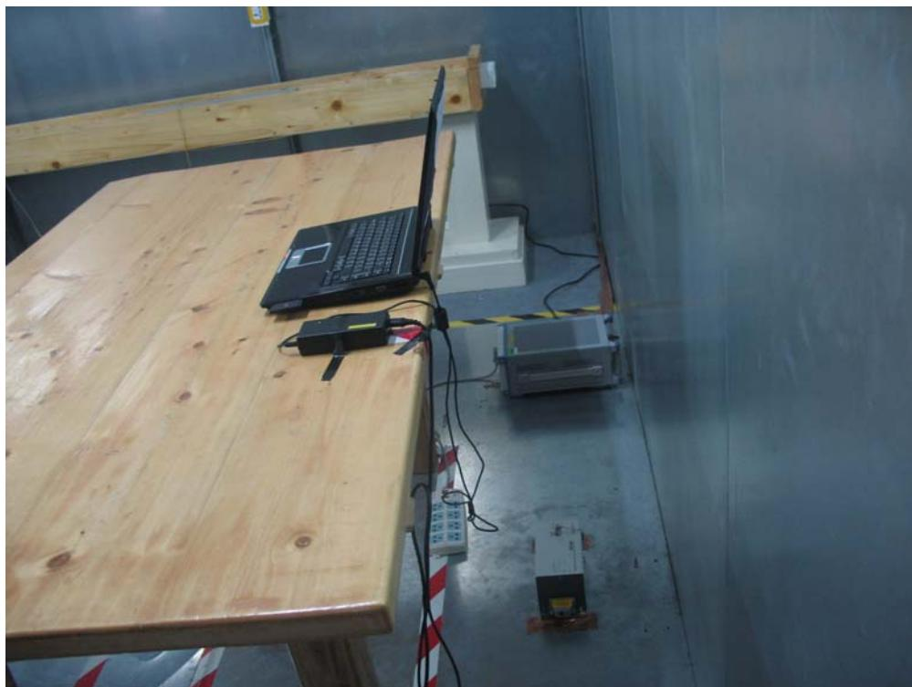
Test Mode: Mode 2: Transmit by 802.11g
