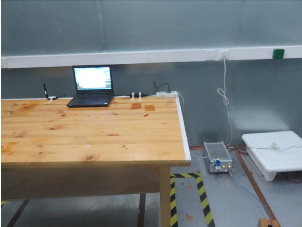
Picture 3 Conducted Emission Test Setup
