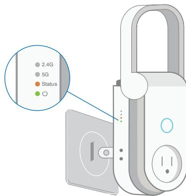
! The Wi-Fi Extender+ must only be installed and operated in an upright vertical position with the antenna pointing upwards.
