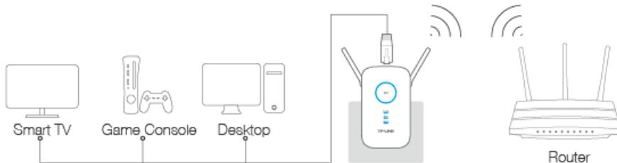
By default, the Ethernet port connects to the 5GHz wireless network. If you want the extender to connect to the 2.4GHz wireless network only, please follow the steps below to finish the settings:
