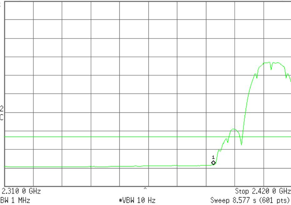
**Band Edges (802.11b / CH High)****Detector mode: Peak**
