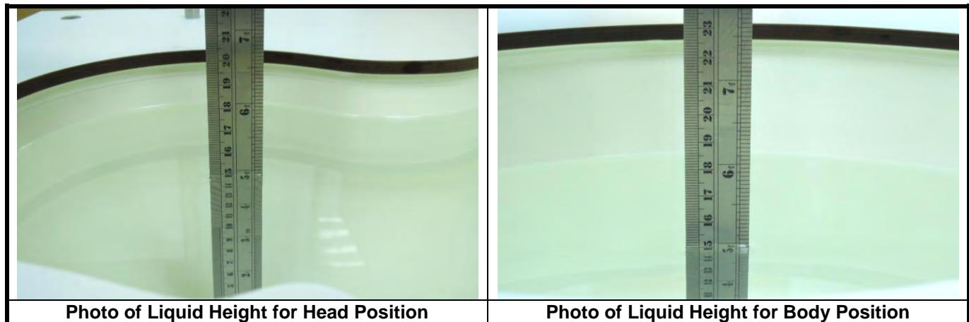
The dielectric properties of the head tissue simulating liquids are defined in IEEE 1528 and FCC OET 65 Supplement C Appendix C. For the body tissue simulating liquids, the dielectric properties are defined in FCC OET 65 Supplement C Appendix C. The dielectric properties of the tissue simulating liquids were verified prior to the SAR evaluation using an Agilent 85070D Dielectric Probe Kit and an Agilent Network Analyzer.
