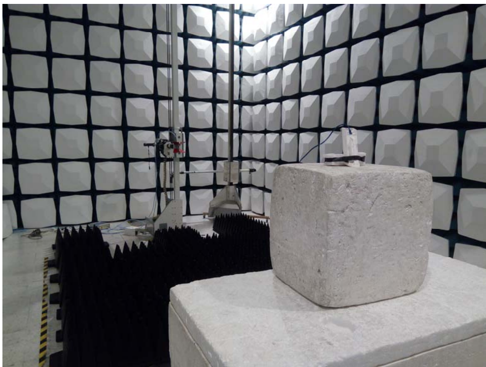
Description: Radiated Emission Test Setup for 1~18GHz
