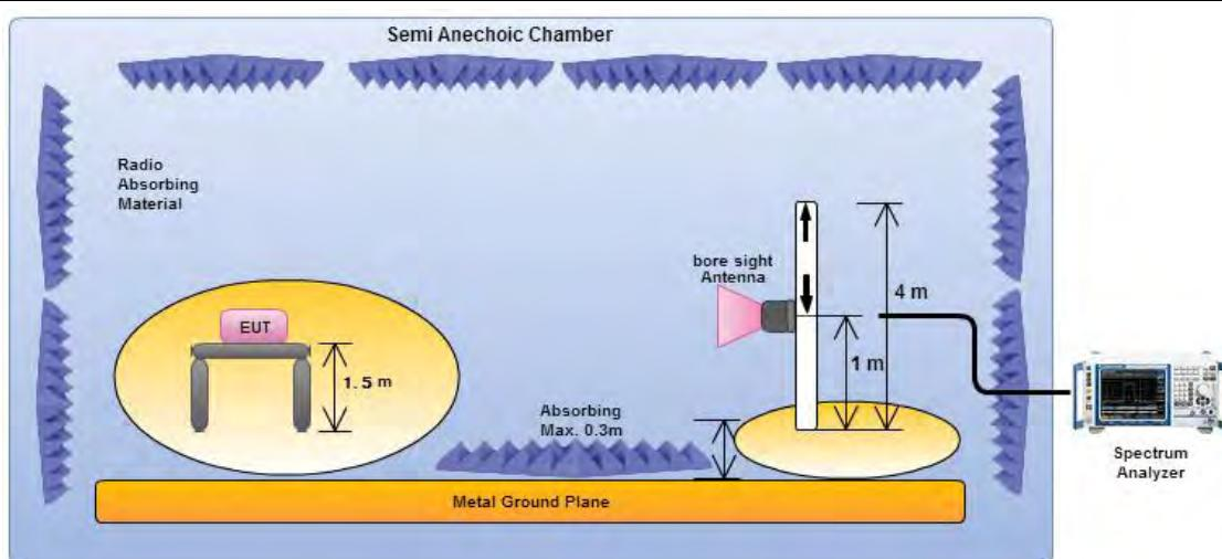
Electric field tests shall be performed in the frequency range of 1 GHz to 10th harmonic of highest fundamental frequency or 40 GHz using a calibrated horn antenna.
