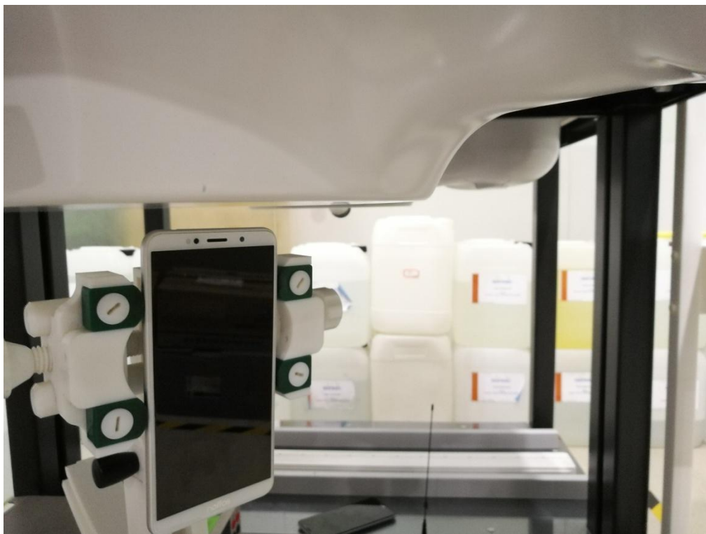
Body top side(separation distance is 10mm)
