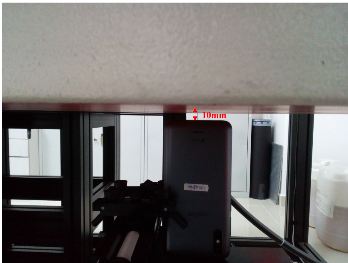
Body Bottom Setup Photo (10mm)
